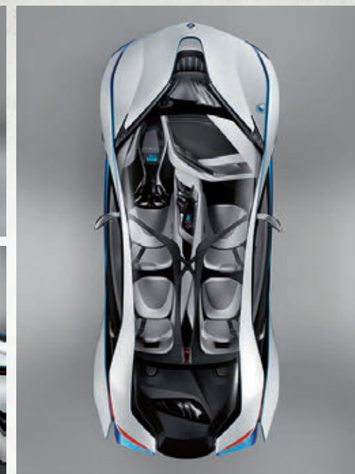
The 2+2-seater study of 2009 previewed today's advanced tapered design, which is aerodynamically based on a droplet of water.
