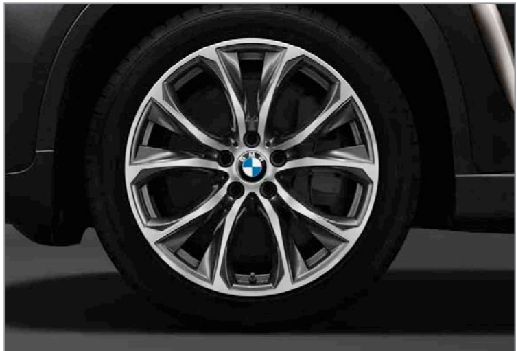
V Spoke light alloy wheels (Style 597) 20 x 10.0 front, 20 x 11.0 rear; and 275/40 front, 315/35 rear run-flat performance tires 1,2,3
