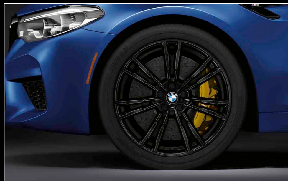
20" M Double-spoke bi-color wheels, style 706M, 20 x 9.5 front, 20 x 10.5 rear; and 275/35 front, 285/35 performance 1,2 non run-flat 3 tires
