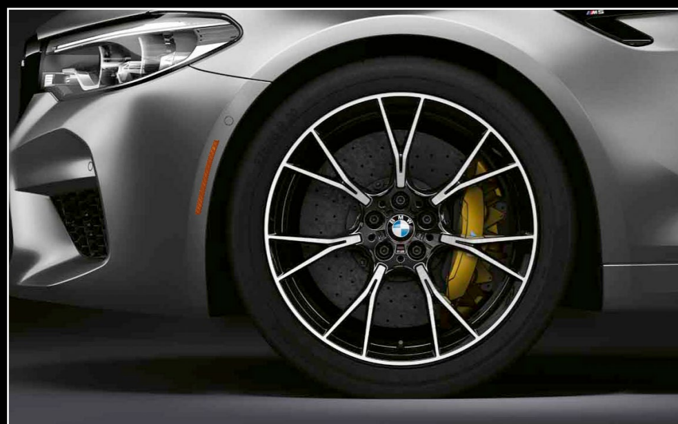
20" M Y-spoke forged bi-color wheels, style 789M, 20 x 9.5 front, 20 x 10.5 rear; and 275/35 front, 285/35 performance 1,2 non run-flat 3 tires
