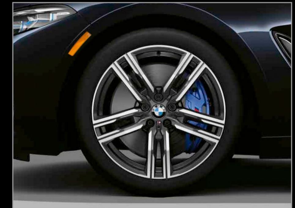
19" M Double-spoke orbit grey wheels, style 727M, 19 x 8.0 front, 19 x 9.0 rear; and 245/45 front, 275/35 rear run-flat 1 all-season tires 2
