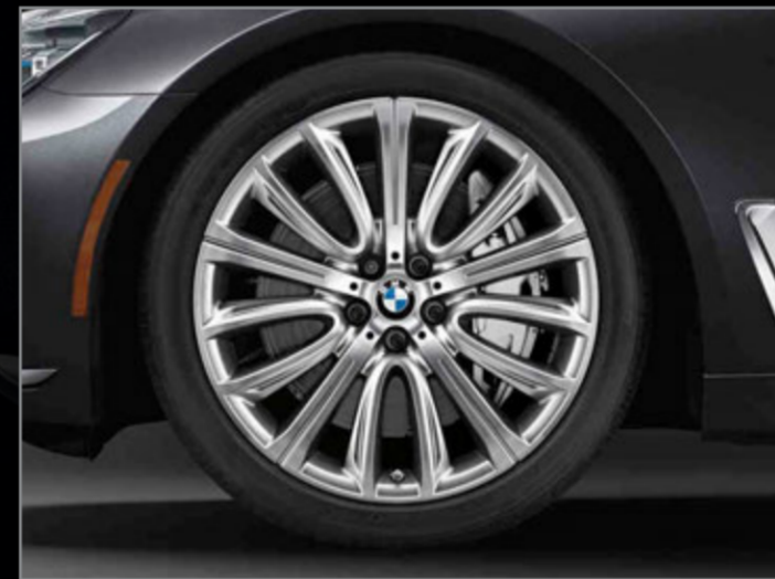
20" V-spoke bi-color wheels, style 628 20 x 8.5 front, 20x10.0 rear; and 245/40 front, 275/35 rear run-flat 1 performance tires 2,3
