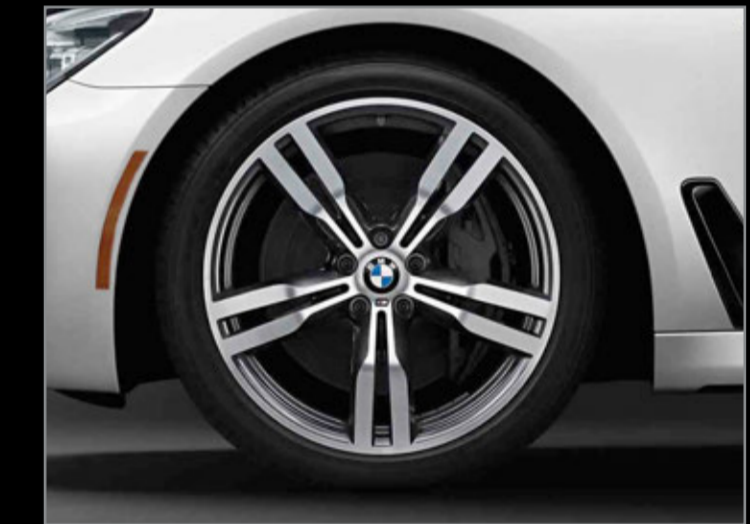
20" M Double-spoke wheels, style 648M 20 x 8.5 front, 20x10.0 rear; and 245/40 front, 275/35 rear run-flat 1 performance tires 2,3
